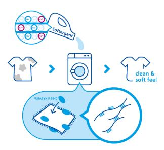
Illustration: Simplified presentation of a wash cycle with a softergent. PURABYK-P 5540 prevents fabric fibers from clogging, making them softer to the touch.
