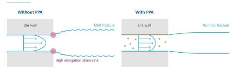
Mode of action of BYK-MAX P 4109 and BYK-MAX P 4110 – Prevention of melt fracture
